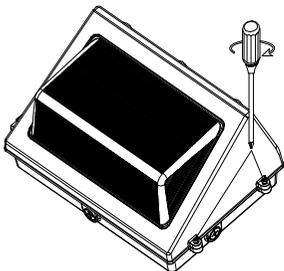
11. Fix the fixture with screws.
