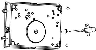
7. Use a screwdriver to remove the side plug and attach the EVA cotton pad to the mounting hole.
