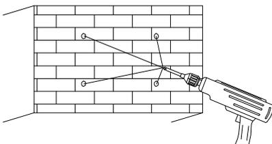
5. Drill a hole in the wall with an electric drill.
