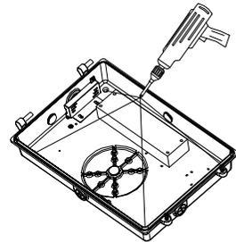
4. Drill through the mounting hole with an electric drill.
