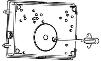
4. Use a screwdriver to remove the plug.
