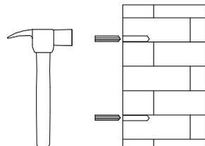
6. Push the expansion rubber plug into the mounting hole on the wall.
