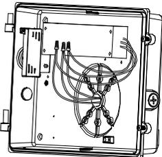
9. Connect L,N and G wires to the power supply
