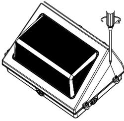
11. Fix the fixture with screws.
